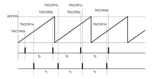
Time intervals can be produced with other modes as well, where TACCR0 is used as the period register. Their handling is more complex since the sum of the old TACCRx data and the new period can be higher than the TACCR0 value. When the previous TACCRx value plus  $t_X$  is greater than the TACCR0 data, the TACCR0 value must be subtracted to obtain the correct time interval.
